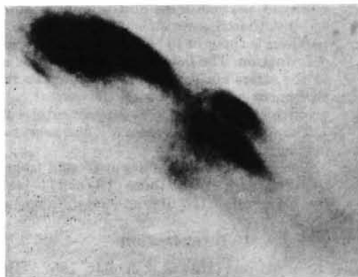
Fig. 2. Enlarged Laue streak from a microbeam photograph of one kink band on the surface of a lightly deformed single crystal of aluminium. Fine parallel striations may be seen running diagonally from the top left hand corner.
